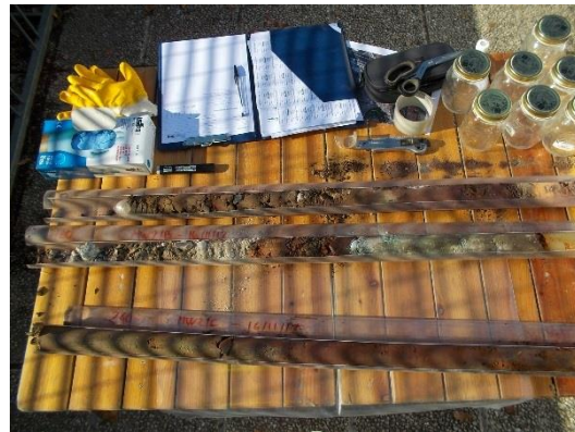
Sondaggio MW2 – carote 0.0-2.4 m
