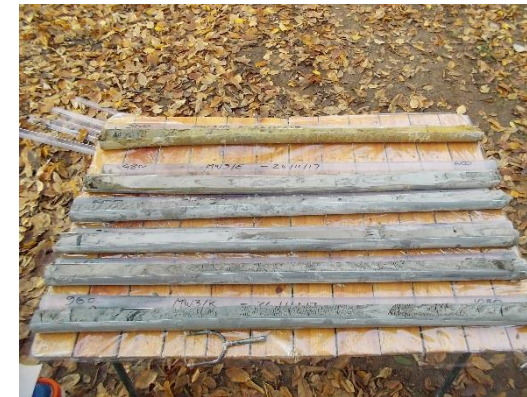
Sondaggio MW3 – carote 3.6-10.8 m
